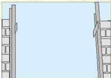
Vertical frame work erected, end secured and horizontal level taken
